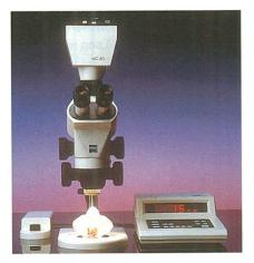
The new Carl Zeiss stereomicroscope Stemi 2000-CS allows the user to view the sample whilst other observers view the procedure by video. Greenough type stereomicroscopes create their
